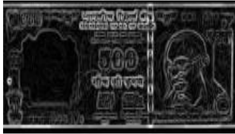
Fig.6 : Edge Detection (Gradient magnitude of the image)
